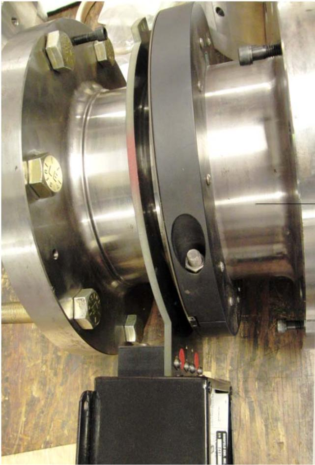
**Note positioning of receiver; roughly a 1/4-to-3/4" gap between the stator ring and rotor ring should be sufficient, but the closer distance would require less power thus more efficient.**
