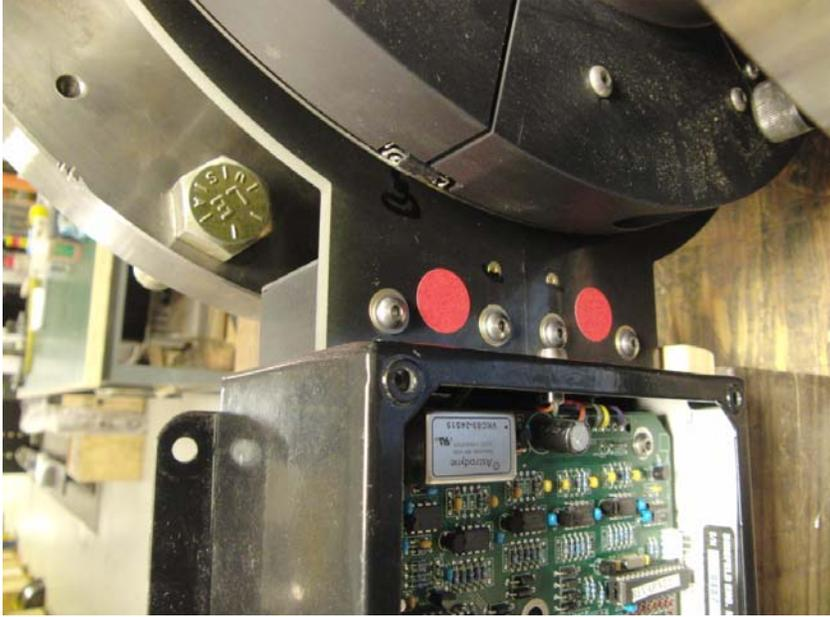
**RED stickers were placed on the side of stator ring that must face the rotor ring.**
